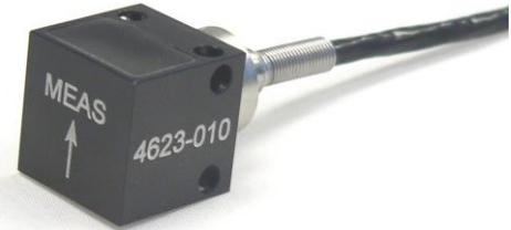
The **Model 4623** is a low frequency DC response accelerometer offering outstanding performance over a wide operating temperature range. The accelerometer is available in ranges from  $\pm 2$  to  $\pm 100g$  and incorporates an EMI/EMC protection circuitry for harsh installations. The output is signal conditioned to provide a low noise amplified signal. The model 4623 incorporates a PFA insulated cable with a rugged strain relief designed for demanding applications.
