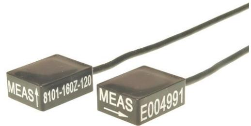
The **Model 8101** is a low cost, plug & play accelerometer designed for general purpose vibration measurements. The accelerometer is available in  $\pm 40g$  or  $\pm 160g$  range and provides a flat frequency response up to  $>6kHz$ . Featuring stable piezo-ceramic crystals in shear mode, the accelerometer incorporates full power and signal conditioning and is offered in two measurement direction options (X or Z axis).
