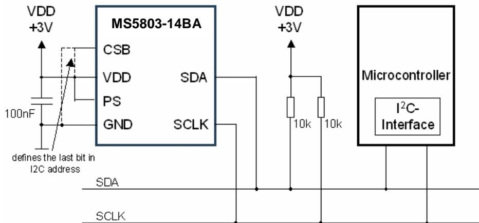
Figure 16: Typical application circuit with SPI / I<sup>2</sup>C protocol communication
