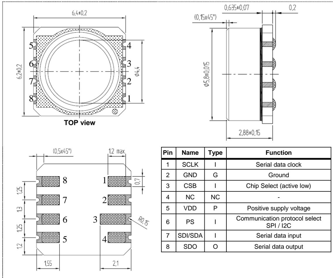
Figure 17: MS5803-14BA package outlines, pin configuration and description
