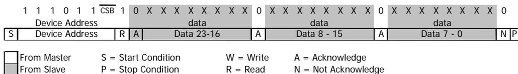
Figure 13: I<sup>2</sup>C pressure response (D1) on 24 bit from MS5803-14BA
