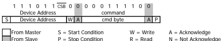
Figure 10: I<sup>2</sup>C Reset Command
