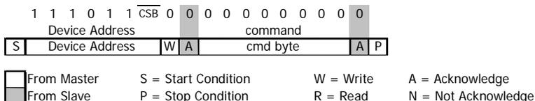
Figure 12: I<sup>2</sup>C ADC read sequence
