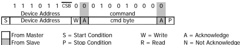
Figure 11: I<sup>2</sup>C Command to initiate a pressure conversion (OSR=4096, typ=D1)
