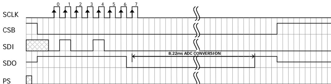
Figure 7: Conversion out sequence, Typ=d1, OSR = 4096
