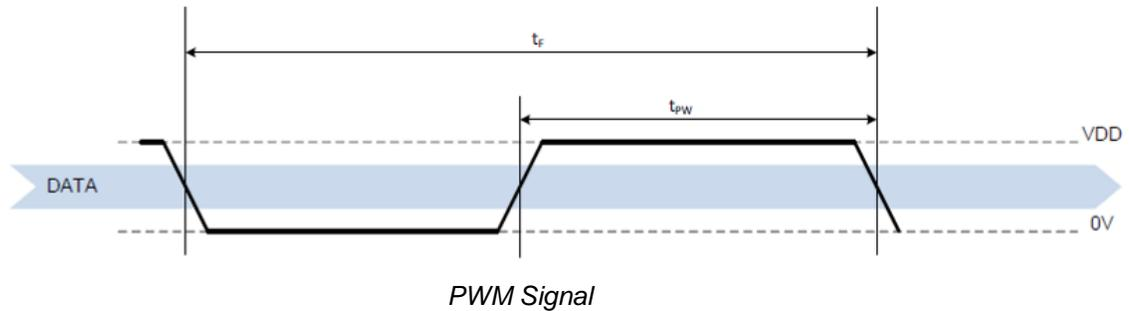
Base frequency runs constantly at approximately 120 Hz, hence  $t_F$  is about 8.3ms. The signal is provided on  $t_{PW}$  as a ratio of  $t_F$ . The measured data – either relative humidity or temperature – is provided as ratio of  $t_{PW}$  and  $t_F$ .  $t_{PW}$  shall always be given as ratio of  $t_F$  to make it independent of variations of the base frequency.
