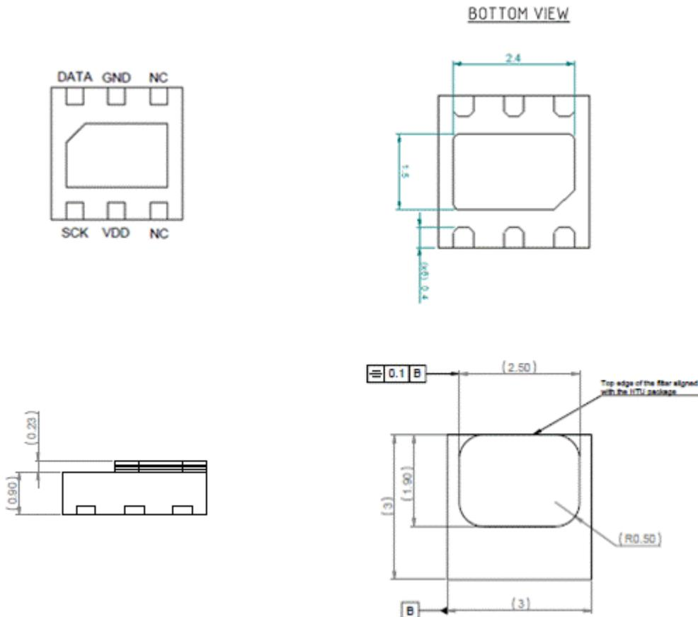
Dimensions are given in mm, tolerances are  $\pm 0.1$  mm. The die pad (thermal center pad) is internally connected to GND.
