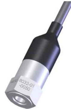
The **Model 8032-01** is an internally shielded rugged IEPE accelerometer designed for harsh environments. The accelerometer is available in  $\pm 50$  to  $\pm 500g$  dynamic ranges and has a flat bandwidth up to greater than 12kHz. The model 8032-01 features an integral molded strain relief and is designed to operating in temperature ranges from -55°C to +125°C. The unit is hermetically sealed and features the popular stud mount installation.
