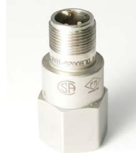
The **Model 8011-01** is an internally shielded rugged IEPE accelerometer designed for harsh environments. The accelerometer is available in  $\pm 80g$  dynamic ranges and has a flat bandwidth up to greater than 16kHz. The model 8011-01 features a top exit MIL-C-5015 connector and is designed to operating in temperature ranges from -55°C to +125°C. The unit is hermetically sealed and features the popular stud mount installation.
