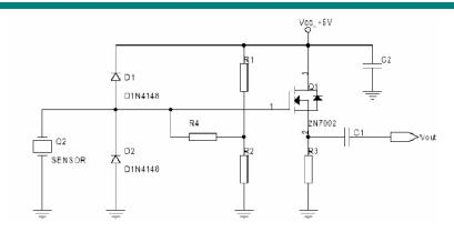
Shield (braid): GND Red wire: V<sub>cc</sub>, +5V Yellow wire: Vout C1 = C2 = 0.1 µF R1 = R2 = 300K R3 = 10K R4 = 100M
